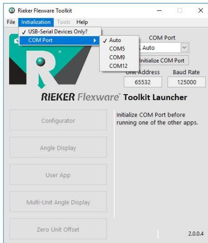
To access and configure the Flex inclinometer, install the Flexware™ Toolkit App, which is provided on the included USB Flash Drive. Connect the USB Interface Cable to the H6, then attach the USB connector to the PC USB port. External power is required, such as an AC/DC 24VDC wall adaptor. The software will detect the sensor, allowing the user to reconfigure the parameters. See the "Flexware™ Software User Guide" for installation and configuration details.
