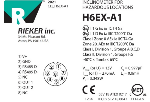
FIGURE 2: Top Surface Markings for H6EX-A1 Showing Hazardous Location Information
